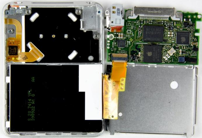
**⚠** The logic board is still connected to the front case by the display ribbon cable, located on the headphone jack side of the logic board.
