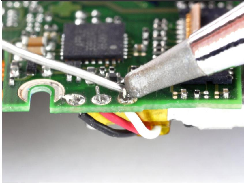
**i** In this step, you will solder the battery leads to the solder pads on the logic board.
